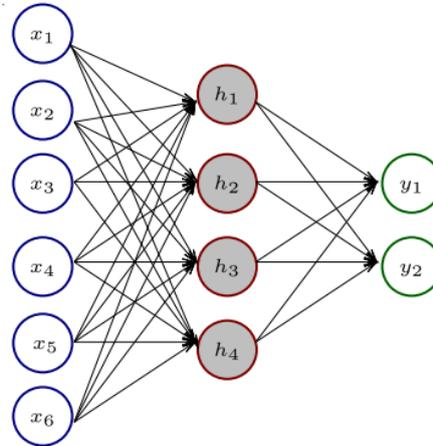
Figure 1: Architecture of neural net topology with 6 input variables, 4 hidden units and 2 outputs.
