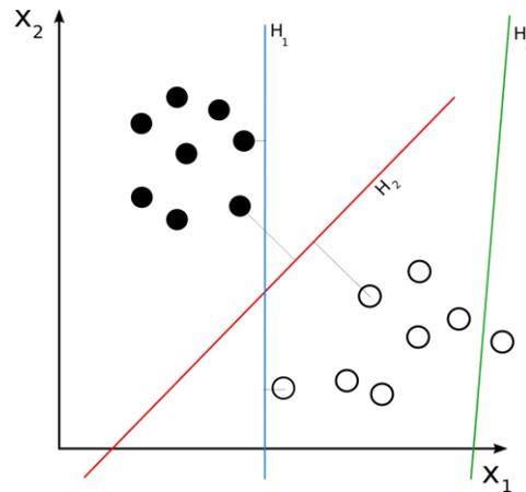
Figure 2: Classification problem using SVM with linear separable case: graphic showing three hyperplanes in two dimensions. H3 doesn't separate the two classes. H1 does, with a small margin and H2 with the maximum margin.
